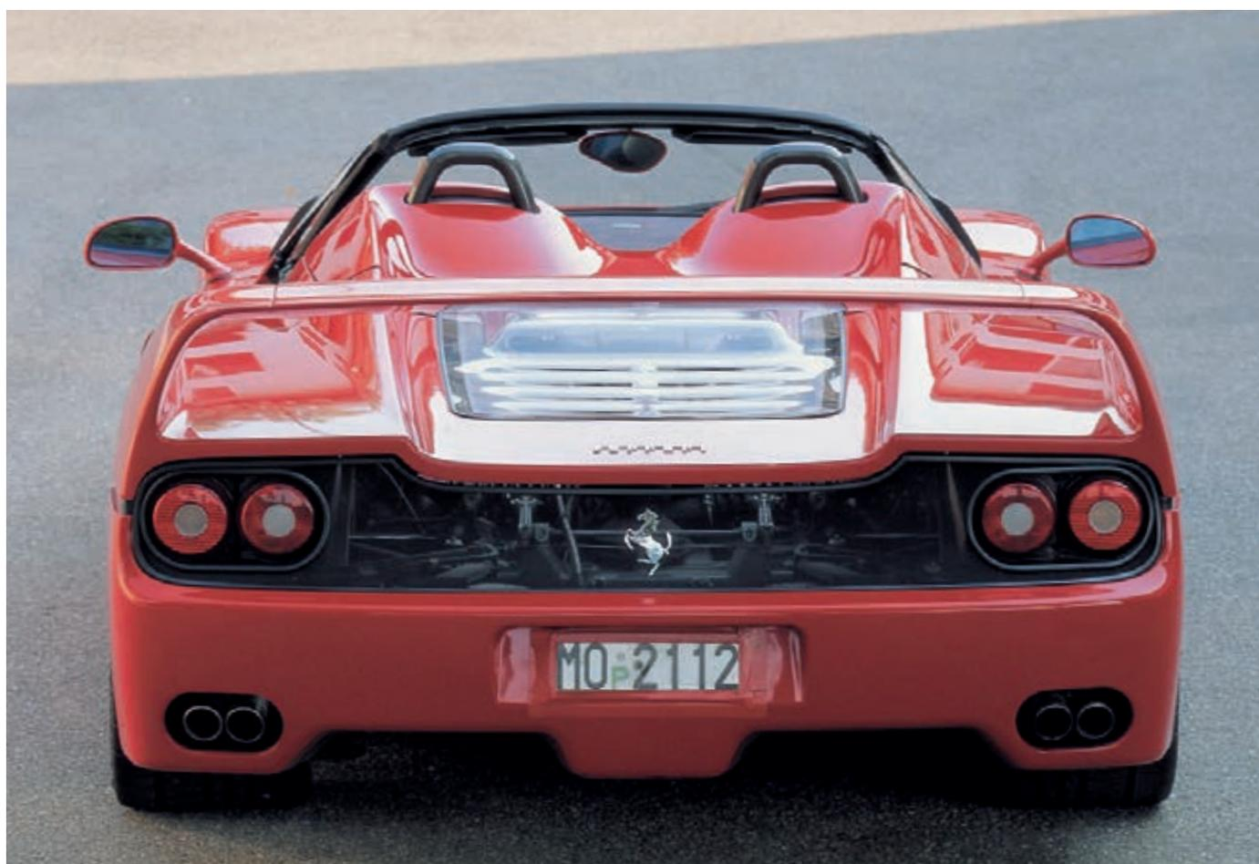
*The F50 seemed to literally suck up the road. Its aerodynamics, optimized in the wind tunnel, produced a vacuum and down force, and ensured that driving was stable even at speeds beyond 200 mph (300 kph).*
